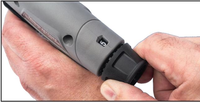
To change the tension setting, pull back the Tension Adjustment Knob, match it to the appropriate cable tie cross section tension setting, and disengage the knob.
